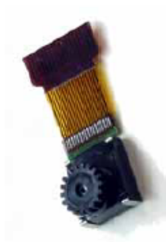
Figure 3: Agilent ADCM-1700 is a CIF resolution ultracompact module that is only 8.0 \times 7.0 \times 5.4mm
