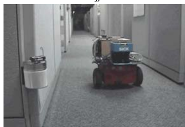
Figure 3: a) Navigation Field produced; b) Example of the path taken; c) An example of a discrete probability distribution of node k for direction (action) "East" (i.e. right); d) Experimental environment with 9 nodes; e) Path taken by the robot from node 1 to node 9; f) Mobile Robot and a Sensor Node during a real world experiment in the environment in d);
